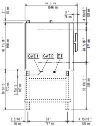
CWII Cold Water inlet 1 CWI2 Cold Water Inlet 2
